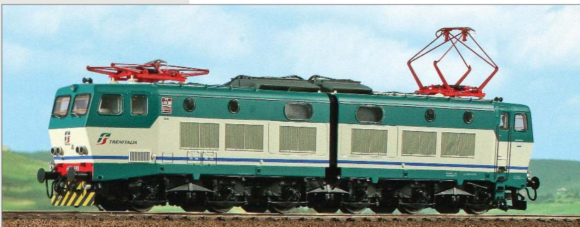
Locomotiva articolata delle FS E.656.598 (sesta serie). Livrea XMPR, pantografi Tipo FS 52, respingenti tondi. E.656.598 Italian Railways locomotive (sixth series). XMPR livery, Type 52 pantographs, round buffers. E-Lok E.656.598 der italienischen Eisenbahnen (sechste Bauserie). XMPR Lackierung, Typ 52 Stromabnehmer, runde Puffer.
