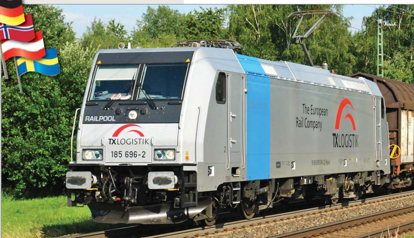
Locomotiva Tipo E 185, livrea TX Logistics. Type E 185 TRAXX locomotive, TX Logistics livery. E-Lok Typ E 185 TRAXX, in TX Logistics Lackierung.
