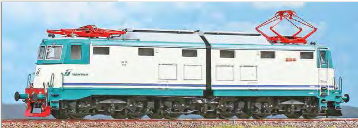
Locomotiva delle FS E.636.429 in livrea XMPR con terzo faro. Deposito di Udine. E.636.429 of the Italian Railways locomotive, XMPR livery with third light. Udine depot. FS-Lokomotive E.636.429 in XMPR Lackierung, mit drittem Spitzenlicht. Bw Udine.
