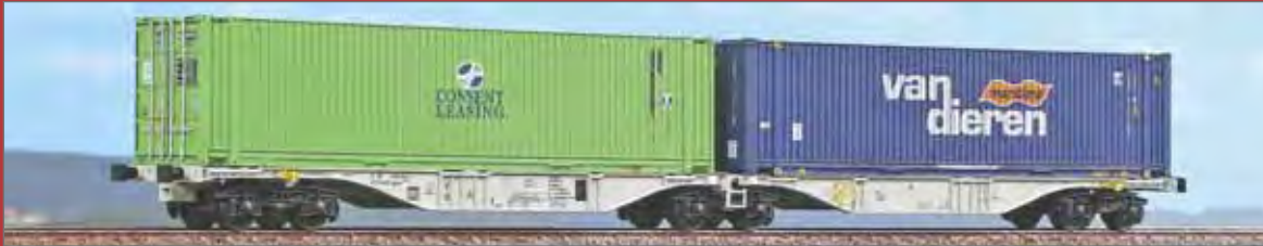
Carro intermodale Tipo Sggmrss '90 bimodulo noleggiato "Hector Rail" con carico di casse mobili furgonate. Container wagon Type Sggmrss '90 hired by "Hector Rail" with swap bodies. Containerwagen Typ Sggmrss '90 Doppelmodul vermietet an "Hector Rail" mit Wechselpritschen.
