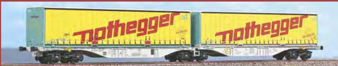
Carro intermodale Tipo Sggmrss '90 bimodulo noleggiato "TX Logistics" con carico di casse mobili. Container wagon Type Sggmrss '90 hired by "TX Logistics" with swap bodies. Containerwagen Typ Sggmrss '90 Doppelmodul vermietet an "TX Logistics" mit Wechselpritschen.
