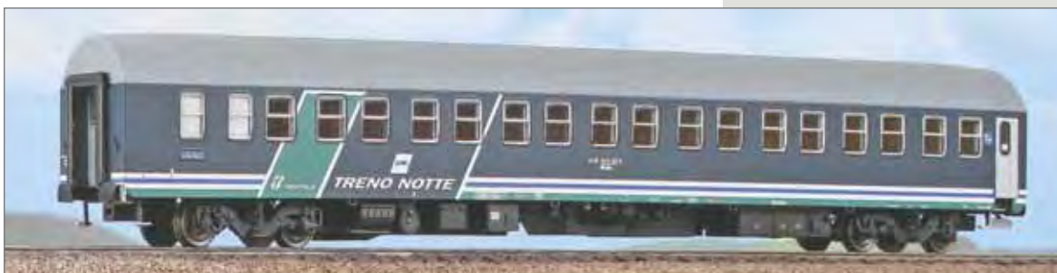
Carrozza letti FS Tipo T2s 1982 con carrelli FIAT, livrea XMPR "Treno Notte". FS Type T2s 1982 sleeping car with FIAT bogies, XMPR "Treno Notte" livery. FS Typ T2S 1982 Schlafwagen mit FIAT Drehgestellen, XMPR "Treno Notte" Lackierung.
