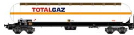
60 140 Uas Totalgaz, blanc, pare soleil, bouts sphériques, Ep.IV-V white, with sun protection, spheric ends Ep.IV-V
